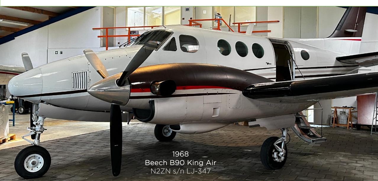
Newly delivered to Volkswagen as D-IEVV in 1968 and since 2008 active under an US registration with the new owner, this King Air is a typical Beechcraft product. This King Air B90 has a 9,650 lb take off gross weight, an increased wingspan and improved instrumentation. This model has the PWC PT6A-20 engines, with a cruise speed of 235 knots, a range of 1,185 nm, and climb rate of 2,000 feet per minute.
